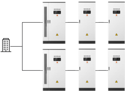
Parallel connection of the hybrid inverter will enable further system expansions.
