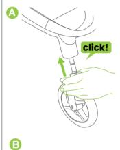
A. Insert each front swivel wheel assembly into the wheel moulding and push in until you hear a 'click'. Pull on each wheel to make sure it is securely attached. Repeat the process if not locked in.
