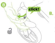
B. To allow the wheels to swivel, slide the lock button to the opposite side until you hear a 'click'.
