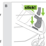
Align the lower second seat adaptors to the frame sockets and press down until you hear a 'click'. Ensure both adaptors are locked in position before attaching the second seat.
