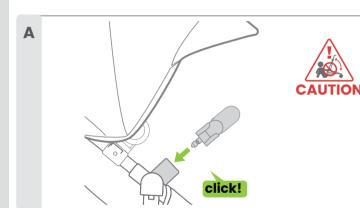
Insert the arm bar mouldings into the sockets on each side of the seat and push in until it locks in position.
