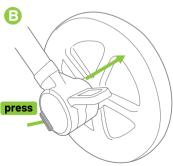
B. To remove the rear wheels, press and hold the release button located under wheel housing and pull away.
