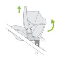
Engage the brake. Pull and hold the release lever on the back of the baby capsule and lift to remove from stroller.
