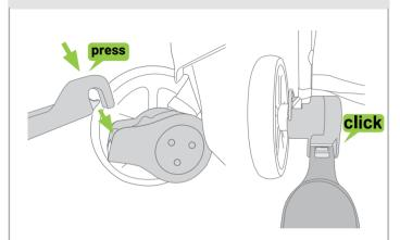
Press and hold the button on the Buggy Board and hook the Buggy Board to the Wheel Hub connector, until it "CLIKS" into place.
