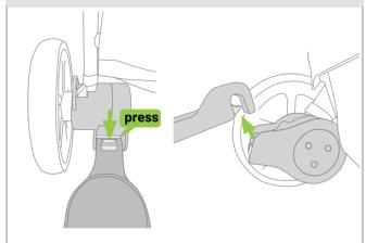
Press and hold the button on the Buggy Board and lift the Buggy Board away from the Wheel Hub connector. You must remove the buggy board before folding the stroller. The wheel hub can remain attached to the stroller.
