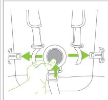
Press the centre of the buckle to release all straps at once.
