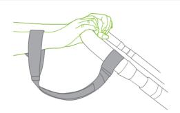
A wrist tether strap is provided on the handle grip. Slide your hand through the tether strap loop whenever you use the stroller. Only remove your hand from the tether strap loop when the brakes have been applied to the stroller wheels.
