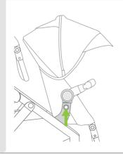
Press both release buttons on the side of the lower adaptors and lift the seat up and away from the stroller frame.
