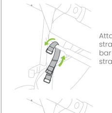
Attach the storage strap to the basket bar by looping the strap over the bar.
