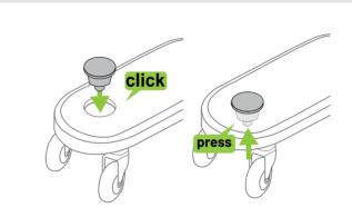
Attach the Buggy Board Cap on the base of the board and cover the seat hole.
