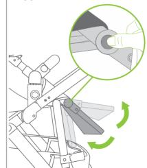
Press and hold the two release buttons on both sides of the leg rest hinge to lower to the desired position. To raise the leg rest simply move it up.
