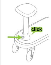
First remove the Cap off the buggy board. Line up the seat with the exposed seat hole and press down until it "CLICKS" into place.
