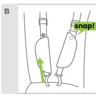
Ensure the shoulder harness pads are secured to the harness strap by using the press studs hidden on the inside of the pads.
