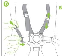
B. Tighten or loosen the waist and shoulder straps by sliding the harness adjuster to the desired fit.
