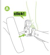
A. Insert wheel axle into the moulding and push in until you hear a 'click'. Pull on each wheel to make sure it is securely attached. Repeat the process if not locked in.
