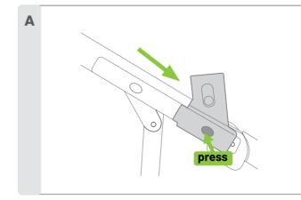
**IMPORTANT:** Ensure the upper seat housing on both sides are adjusted to the lowest seat position for single mode use.
