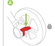
A. Push down the brake pedal to engage the brake.
