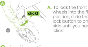
wheels into the fixed position, slide the lock button to one side until you hear a 'click'.
