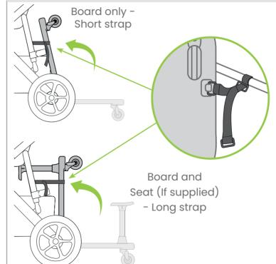
To stow the Buggy Board, rotate it upwards and attach the strap to the appropriate notch on the underside. Use the long strap if the seat is attached, and the short strap if there is no seat.
