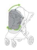
B. To expose mesh window, lift the top cover flap and secure with toggle and elastic loop at the top.
