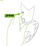
B. To remove the front wheels, push the release button located at the back of the moulding.
