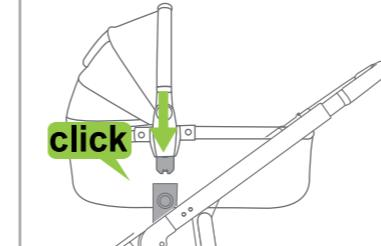
Align the bassinet connectors directly over the seat frame sockets and push down until both connectors lock in place.
