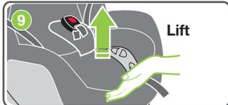
Step 9. Check if the CLICKTIGHT™ frame is locked by gently lifting as shown.
