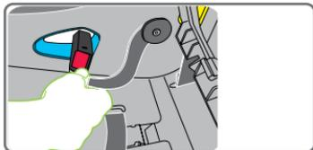
**Step 9.** Store the ISOFLEX® Connectors by engaging each connector into its storage pin. Store the adjuster and indicator under moulding. Tuck in excess ISOFLEX® straps.
