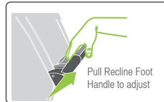
B. Determine whether an upright or reclined position is preferred and adjust if necessary. To adjust the restraint to the fully upright position, grasp the handle on the foot, then pull the handle outwards and hold to release the lock. Rotate the foot fully downwards, then release the handle to lock the foot in the fully upright position. The indicator on the side of the restraint identifies the forward facing and reclined positions.
