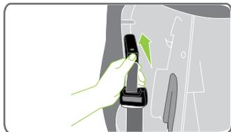
Remove slack but do not tighten. The storage pin may be damaged if the strap is tightened.
