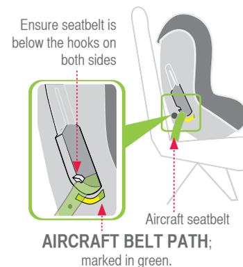
Aircraft label is located on the back of the restraint and demonstrates suitability for use on an aircraft.
