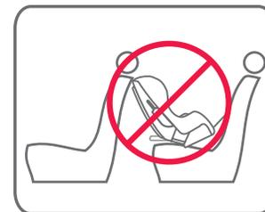
Do not allow the front seat to alter the installed angle of the restraint. It is permissible to allow the restraint to touch the front vehicle seat.
