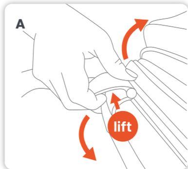
**A** Lift the recline lever on the back of the seat and hold while raising or lowering the backrest to the desired position.
