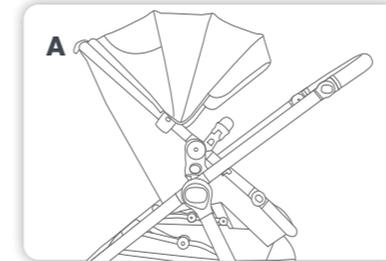
**A** Put the stroller seat into reverse facing position.
