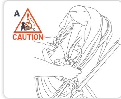
**A** Place the canopy on the stroller seat and push the clips on the sides of the canopy onto the stroller seat until they snap into place.
