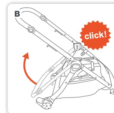
**B** Lift the handle upwards until the frame is fully open and locked.
