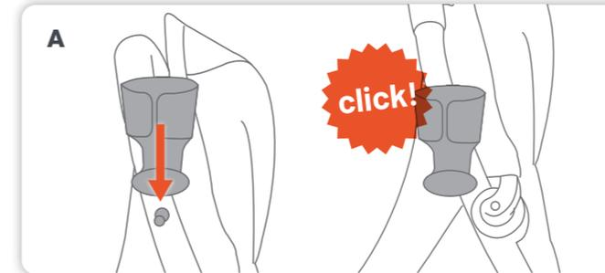
**A** The cup / bottle holder can only fit on the right-hand side of the frame. Push the cup / bottle holder attachment to the connector on the frame.
