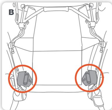
**B** Line up the second seat connectors to the second seat frame socket inside of the stroller frame (located on inside of the rear wheel housing).
