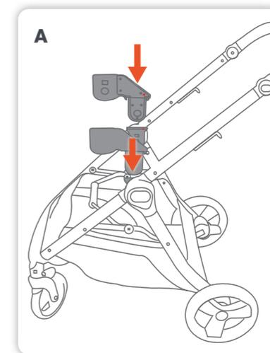
**A** Select the extension adaptor that has a coloured dot and align with the coloured dot on the frame socket. Note: Coloured dots are only on one side of the frame socket. Firmly press down on the Extension adaptor until you hear a 'click' and a green indicator can be seen through a window in the frame socket. Repeat on the other side with the receiver with no coloured dot. To ensure the receiver is engaged pull upwards.
