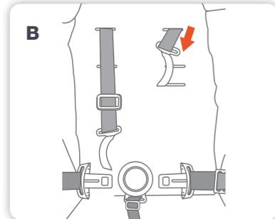
**B** Select the appropriate shoulder harness height and pull each shoulder harness tongue through the harness slot.
