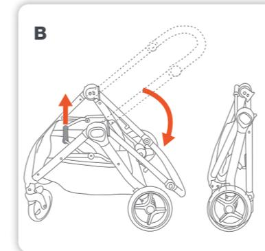
**B** Pull the handle under the stroller seat upwards until you hear a 'click' and the frame is fully folded and the frame lock latch is locked in properly.
