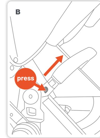
**B** To remove the arm bar, press the button on each side of the arm bar moulding and pull arm bar up and out of the sockets.
