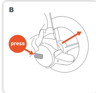
**B** To remove the rear wheels, press and hold the release button in the wheel housing and pull away.
