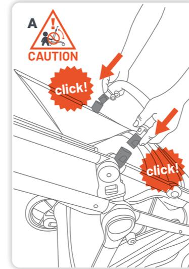
**A** Insert the arm bar mouldings into the sockets on each side of the stroller frame and push down on the arm bar until a 'click'.
