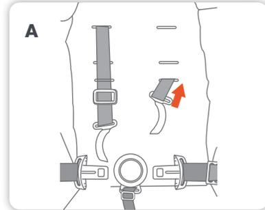
**A** To change the shoulder harness height, push the shoulder harness tongue out of the current harness slot and through the back of the seat.
