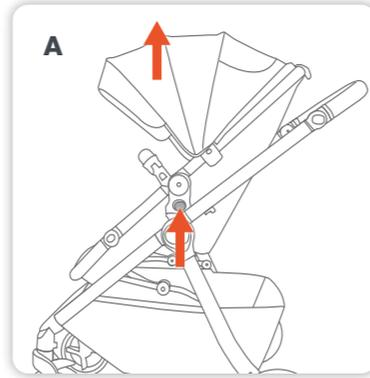
**A** Lift both release levers on the seat connectors at the same time and lift the seat up and away from the stroller frame.
