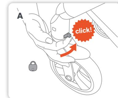
**A** To lock the front wheels into the fixed position, slide the swivel wheel locking clip towards the inside of the frame until you hear a 'click'.
