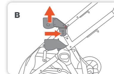
**B** To remove the extension adaptors, press in and hold the button on the inside of the receiver and pull up the extension adaptors out of the frame sockets.
