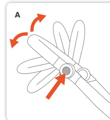
**A** Press the two release buttons on the outside of the handle and hold while raising or lowering the handle to the desired position. When the desired height has been achieved let go of both release buttons.
