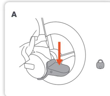
**A** Push down the brake pedal to engage the brake.
