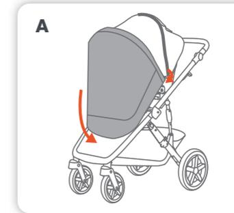
**A** Fit the sun shade over the canopy front and secure the toggle and elastic loop around the canopy frame then pull to the front and secure with the elasticised end.
