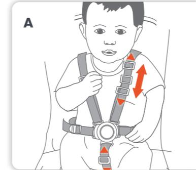
**A** Tighten or loosen the shoulder straps and crotch strap by sliding the harness adjuster up or down. The crotch strap should be adjusted to a snug fit.
