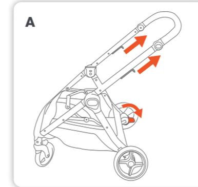
**A** Engage the brake. Pull the latches on the handle tube upwards and drop down the handle all the way.
