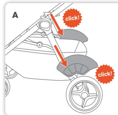
**A** Slide each guard onto the mounting bracket above each rear wheel housing and push down until it locks into place. There is left and right wheel guard. Please ensure it is locked.
