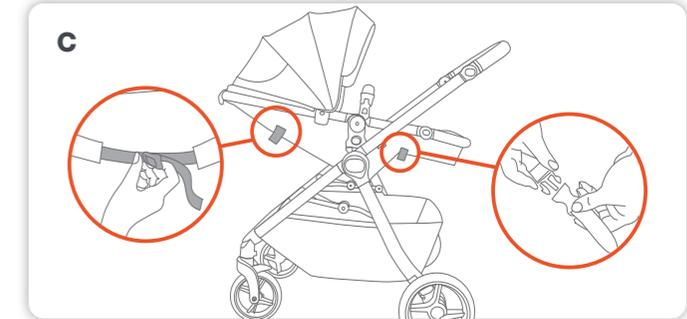
**C** Pull the backrest clip to extend the strap all the way and push down the backrest. Unbuckle the clip under leg rest and push down the leg rest.
