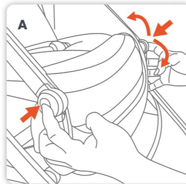
**A** Press the two release buttons on both sides of the leg rest hinge and hold while raising or lowering the leg rest to the desired position.
