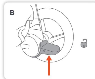
**B** Push the brake pedal upward until the brake is disengaged.
