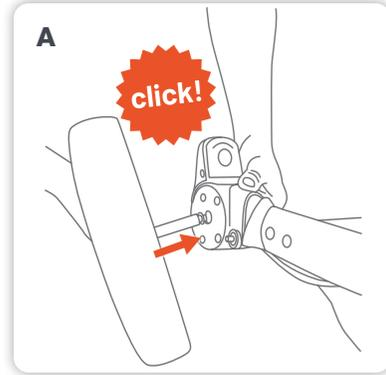
**A** Insert wheel axle into the moulding and push in until you hear a 'click'. Pull on each wheel to make sure it is securely attached. Repeat the process if not locked in.
