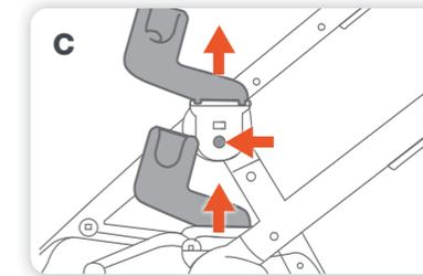
**C** To remove the adaptors, press in and hold the button on the bottom of the adaptors then pull up and out of the frame sockets.
