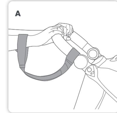
**A** A wrist tether strap is provided on the handle grip. Slide your hand through the tether strap loop whenever you use the stroller. Only remove your hand from the tether strap loop when the brakes have been applied to the stroller wheels.
