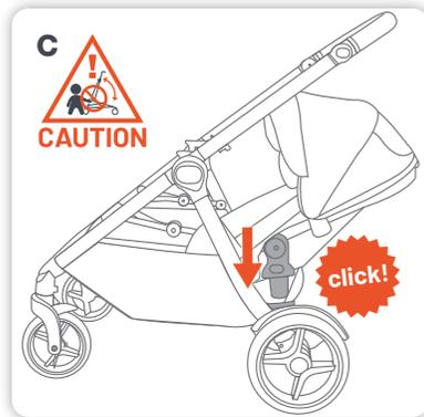
**C** Push down the second seat until it locks. Pull up on both sides of the seat to ensure the seat is locked.
