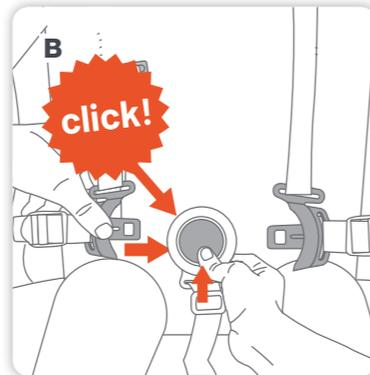
**B** Hold the centre button in on the crotch buckle and insert the waist buckle tongues into the crotch strap buckle until you hear a 'click'.
