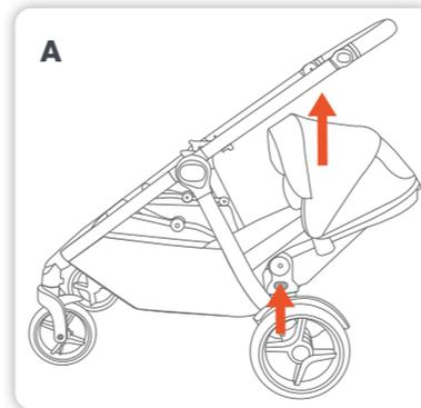
**A** Lift both release levers on the seat connectors at the same time and lift the seat up and away from the stroller frame.
