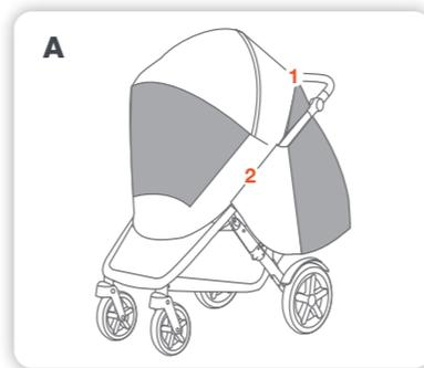
**A** Attach the rain cover extension as required and secure to the rain cover with the zipper (1) and hook & loop (2) attachments.
