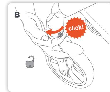
**B** To allow the wheels to swivel, slide the black swivel wheel locking clip towards the outside of the frame until you hear a 'click'.
