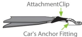
G. Tighten adjustable top tether strap by pulling adjustment strap to remove slack as shown below, but do not over-tighten causing the restraint base to lift off the vehicle seat.
