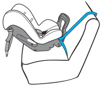
**NOTE:** Seatbelt extenders should not be used if the seatbelt is not long enough to secure the child restraint. If they are used then the buckle must not enter the seating zone.
