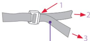
Pull Adjustment Strap to remove slack
