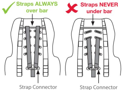
Shoulder straps **must** be threaded through appropriate shoulder strap slots then **over the top** of bar at rear of restraint.
