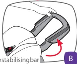
C. While in position, push down on the stabilising bar to lock into position as shown.
