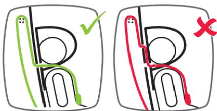
Shoulder straps **must** be threaded directly through appropriate shoulder strap slots then **over the top** of bar at rear of restraint. Harness straps must never be routed through headrest and shell slots at similar heights.
