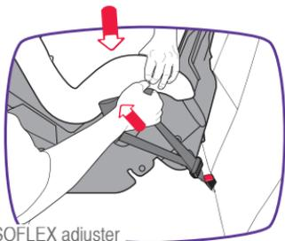
Pull ISOFLEX adjuster strap to tighten
