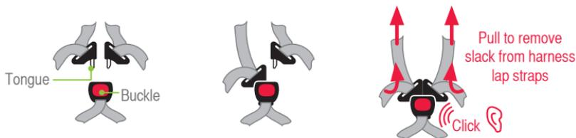
G. Ensure slack is removed from harness lap strap by pulling shoulder straps then pull harness adjustment strap to adjust harness to a comfortable but firm fit. Ensure that any slack in harness straps is removed. Shoulder harness straps must fit firmly to the child. A loose harness could result in serious injury in an accident. Do not over tighten.
