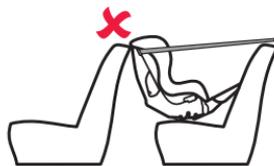
Do not allow the front seat to alter the installed angle of the restraint. It is permissible to allow the restraint to touch the front vehicle seat.
