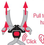
Pull to remove slack from harness lap straps
