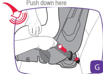
Pull ISOFLEX adjuster strap to tighten
