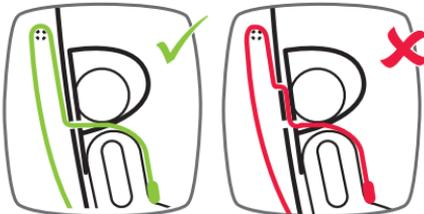
Shoulder straps **must** be threaded directly through appropriate shoulder strap slots then **over the top** of bar at rear of restraint. Harness straps must never be routed through headrest and shell slots at similar heights.
