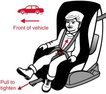
C. Fit either harness tongue into the harness buckle followed by the other tongue until a click is heard. Should the second tongue not insert, press the red button and reinsert the tongues. Ensure secure engagement by pulling harness straps.
