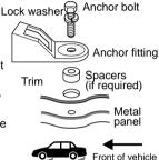
If the car is not fitted with child restraint anchorage points...
