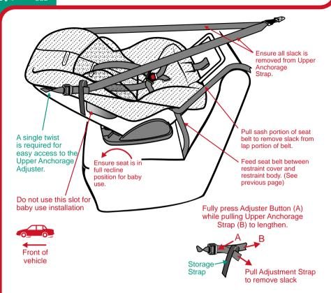
Note: Seat belt buckle and tongue must not rest between restraint cover and restraint. If the seat belt buckle is adjustable, adjust the buckle as low as possible away from the restraint.
