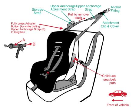
J. Tighten Adjustable Upper Anchorage Strap by pulling adjustment strap to remove slack as shown below, but do not over-tighten causing the restraint base to lift off the vehicle seat. Fold up excess strap and use storage strap to neatly store excess strap away from child's reach.
