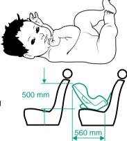
In certain vehicles, where the rear seat area is too restricted, the only position possible for the restraint is on the front seat and adjusted as rearward as possible (provided no airbag is fitted in this position).
