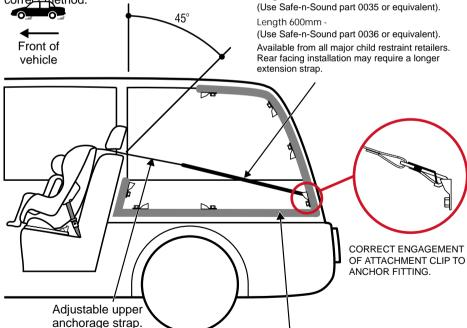
The shaded areas of this diagram illustrate the possible locations of the anchor fitting. Within each shaded area is an anchor fitting showing the correct way to install the fitting. Ensure the anchor fitting is aligned as illustrated unless stated otherwise in the vehicle owner's handbook.
