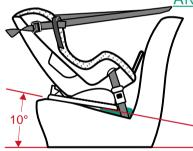
Some vehicle seats have more rearward slope than others. If the angle of the seat causes the baby to be too upright for comfort, the angle may be altered by placing a firm packing between the seat and the underside of the base. Packing can be a firmly rolled up towel or nappy.
