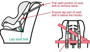
Ensure Harness straps are between restraint moulding and vehicle seat belt.
