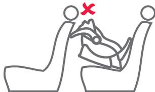
Do not recline the seat excessively, it must be installed at the correct angle (see page 21 - 22).
