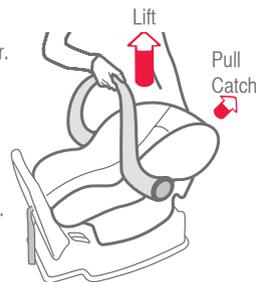
**Always ensure the handle is locked in position before lifting.**
