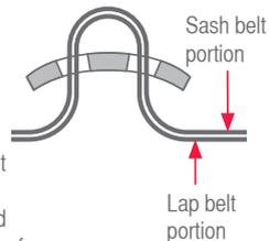
Use this seat belt configuration to install the child restraint according to the instructions on pages 27 to 28. Remove all slack in the lap belt to ensure the base is held firmly against the seat back. This may require adjustment of the strap through the gated 3-bar slide.
