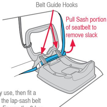
If the seat belt will not stay tight in every day use, then fit a gated 3-bar slide (not supplied with seat) to the lap-sash belt to prevent loosening. See pages 54 and 55. Ensure the 3-bar slide is removed when the Baby Capsule base is not installed to allow other uses to use the seatbelt as a lap-sash seatbelt.
