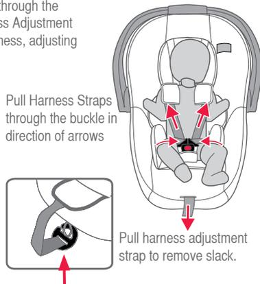
Pull Harness Straps through the buckle in direction of arrows
