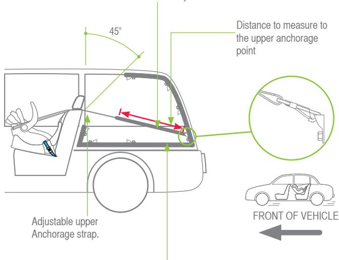
The shaded areas of this diagram illustrate the possible locations of the upper anchorage point. Within each shaded area is an upper anchorage point showing the correct way to install the fitting. Ensure the upper anchorage point is aligned as illustrated unless stated otherwise in the vehicle owner's handbook.
