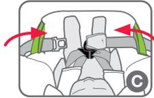
Ensure lap belt is under the hook on each side
