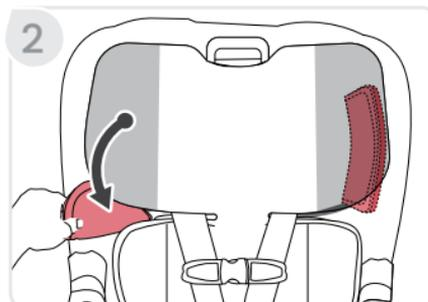
3. **Pull** forward the cover and **route** the harness pad to the front of the head restraint cover. Repeat on the other side.
