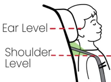
**IMPORTANT:** Harness pads **MUST** be used with children weighing 22- 65 lbs (10 – 29.4 kg) forward-facing except for lap belt only (Type 1) forward-facing installation the harness pads must be stored for children under 25 lbs (11.3 kg).
