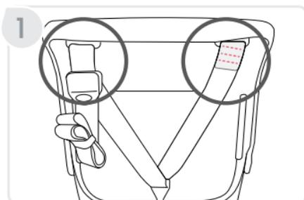
Figure 2 shows an example of when the tether has been damaged and is unacceptable for continued use. If any of the colored stitching has ripped, the child restraint is no longer acceptable for use.
