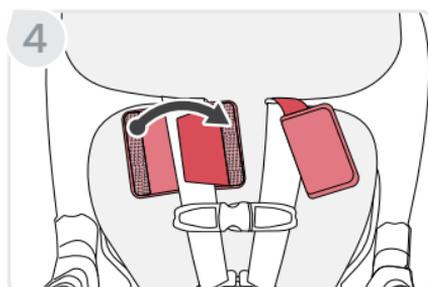
**Note:** Make sure the rubber surface is facing against the child and the strap is not twisted.
