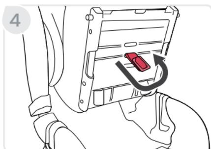
5. **Route** the buckle strap through the desired position and **pull** the buckle strap retainer completely through the seat pan cover and seat pan slot.
