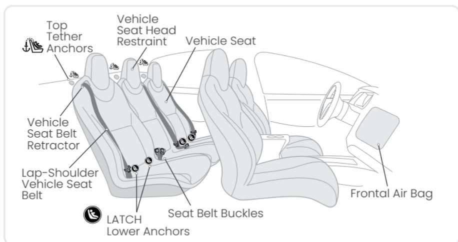
The Lower Anchors and Tethers for Children or LATCH, is a system available on this child restraint that offers an alternative to vehicle belt installation methods. The figure above shows typical locations for lower anchors and tether anchors in a vehicle. See page 2 -3 for LATCH components on this child restraint.
