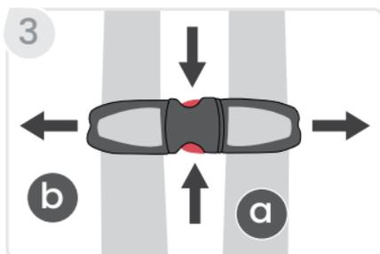
4. **Release** the buckle and the harness straps. **Place** the harness straps to the side.
