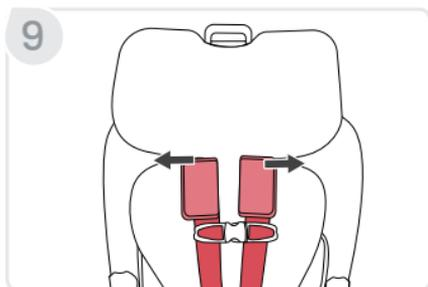
9. **Remove** the head restraint cover.
