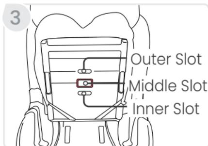
4. **Turn** the buckle strap retainer sideways and **push** it through the seat pan slot and the seat pan cover.
