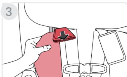
4. **Tuck** the harness strap under the internal harness pad flap and then **fasten** the harness pad around the harness strap. Repeat on the other side.
