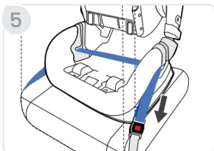
6. **Lock** and remove slack from the vehicle belt.
