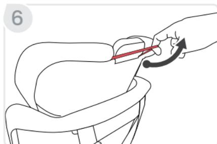
7. **Remove** the two (2) elastic straps from the back of the head restraint. Repeat on the other side.
