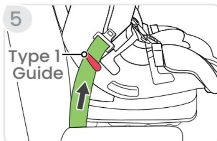
**IMPORTANT:** Do NOT route vehicle belt through BOTH Type 1 guides. Only the guide opposite the vehicle buckle should be used.
